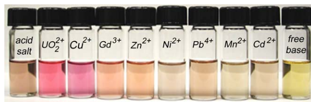
Fig. 12. Colors of \text{MeOH-CH}_2\text{Cl}_2 (95:5 v/v) solutions of isoamethyrin ( 1.02 \times 10^{-4} \text{ M} ) containing four equivalent of \text{Et}_3\text{N} . Acetate salts were used for this study, with the exception of \text{Cd}(\text{NO}_3)_2 [77].
